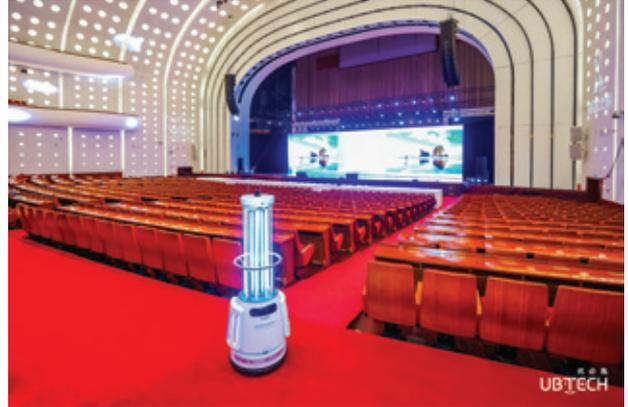
UBTech's ultraviolet disinfection robot, AIMBOT
